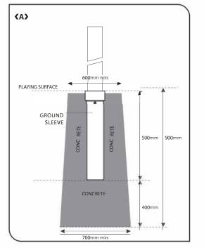
NOTE: Recommended foundation sizing only. Actual foundation depends on local ground conditions.
